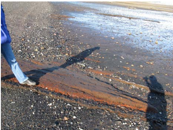
Photo 3-3. Parallel layers, dipping seaward, of hard geochemical iron "cement" (ferricrete), apparently representing past, relatively stable interfaces between the waste rock and the ocean (and between ARD and neutralizing seawater).
