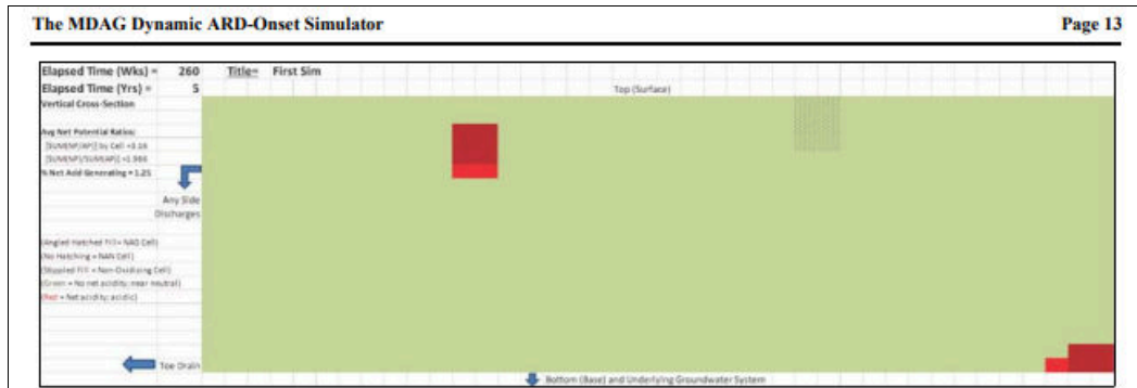
Figure 2-6. After five years, the acidic NAG cells have generated and released sufficient net acidity that NP in adjacent NAN cells has been consumed and they too have become acidic; these NAN cells, if any AP is left, become net acid generating themselves, and release additional acidity to adjacent cells.
