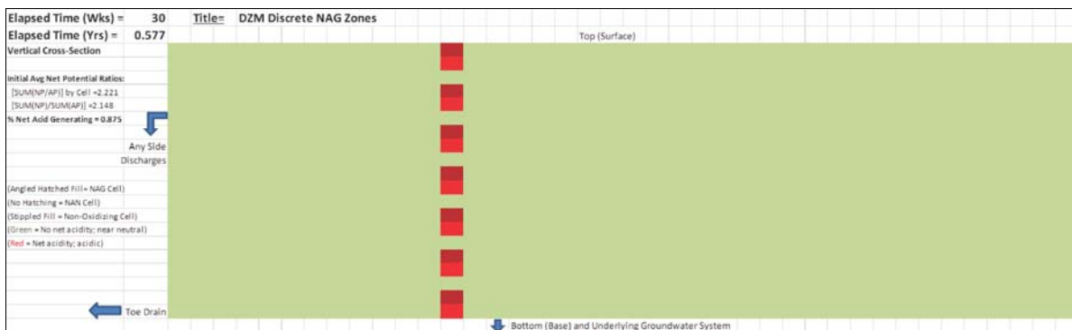
Figure 3-9. Simulation of a vertical stack of NAG cells, each separated by two NAN cells - Week 30; showing the onset of acidic conditions in the NAG cells and in the NAN directly beneath.
