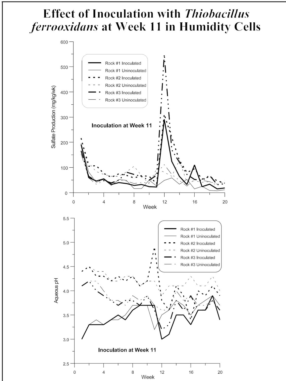
**FIGURE 1. Example of Short-Term Effects from Inoculating Humidity Cells with *Thiobacillus ferrooxidans*.**
